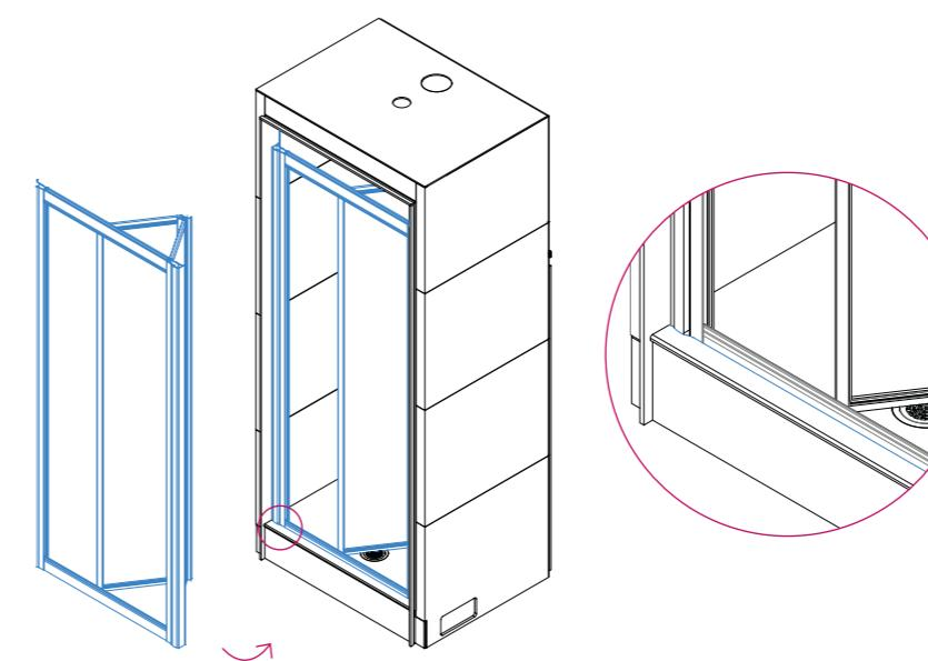
NOTE: Manufacturer's guide may show the door resting on top of step. For the Taplanes cubicle, ensure that door is resting on the floor or door supports.
