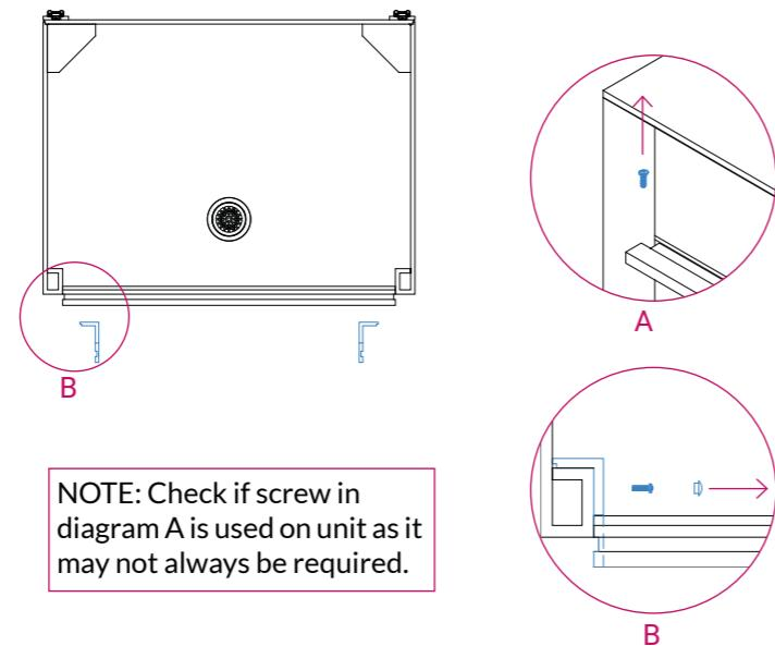
3. Separate soap dishes by removing cover caps and screws.
