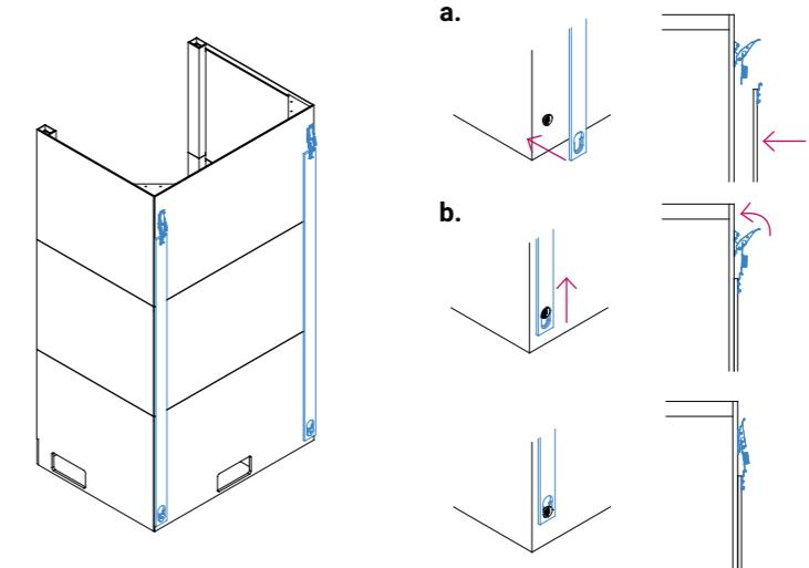
Attach  $\frac{3}{4}$  aluminium backstraps if applicable.
