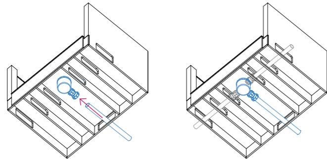
2. Position the base and check level (usually achieved with levelling compound or packers).
