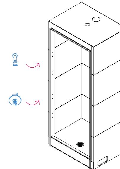
10. Refer to manufacturer's instructions to fit door. Adjust door position to ensure that shower door profile follows step profile.
