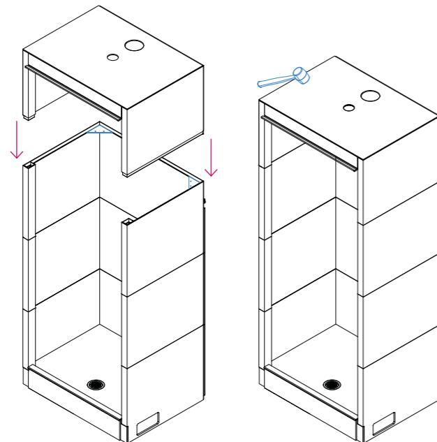
7. Secure top and last middle section by joining soap dishes with screws and fit cover caps.
