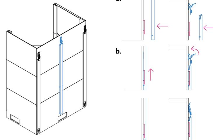
6. Slot in top section and secure with mallet.
