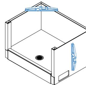
3. Slot in 1<sup>st</sup> middle section and secure with tapping tool and mallet.
