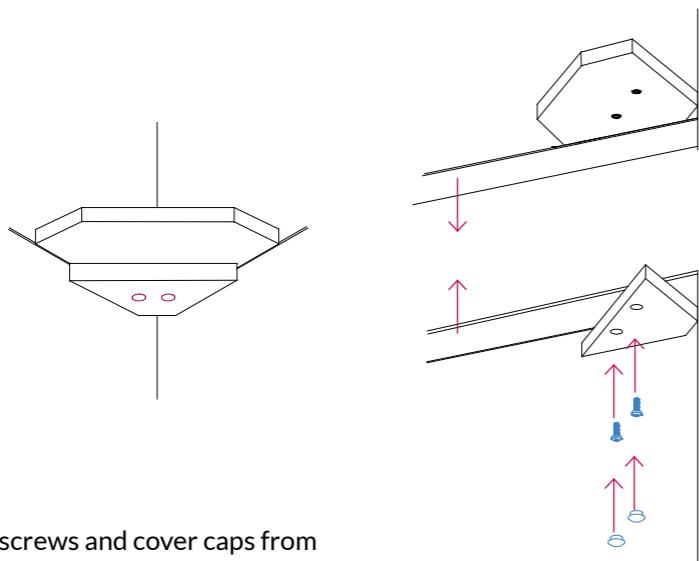
8. Fit side fascias and fix with screws and cover caps from envelope. Be sure to also use previously removed screws. Note the screws on top fascia must also be used.
