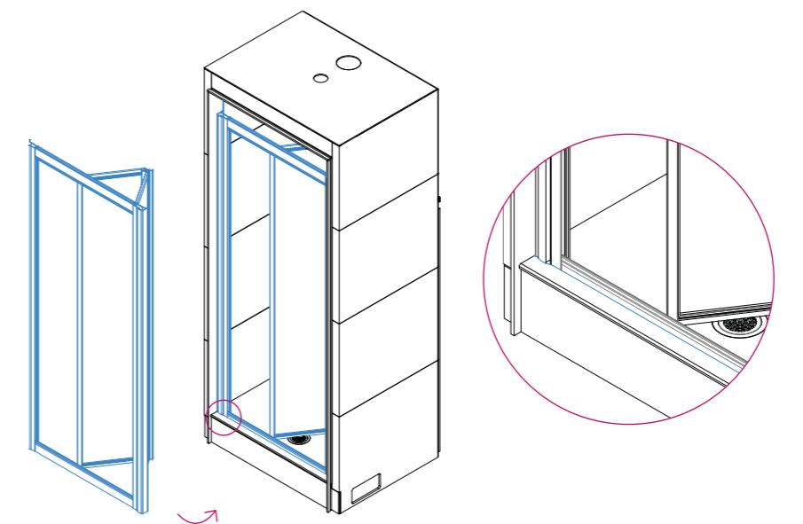
NOTE: Manufacturer's guide may show the door resting on top of step. For the Taplanes cubicle, ensure that door is resting on the floor or door supports.
