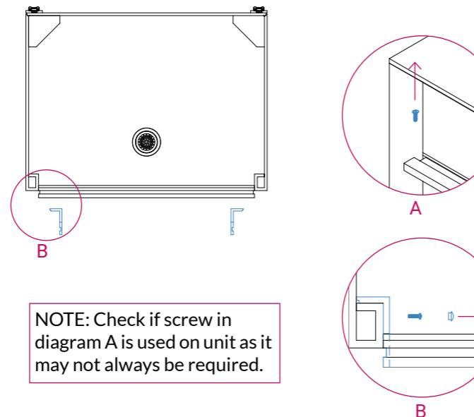
3. Separate soap dishes by removing cover caps and screws.
