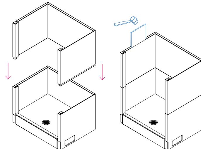
4. Slot in 2<sup>nd</sup> middle section and secure with tapping tool and mallet. Repeat with 3<sup>rd</sup> and 4<sup>th</sup> middle section if applicable.
