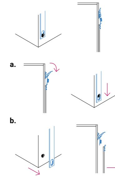
2. Take off door by removing screws connecting door hinges to side fascias.
