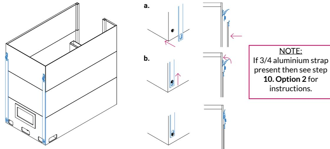
8. Fit side fascias and fix with screws and cover caps from envelope (also using previously removed screws). Note the screws on top fascia must also be used.
