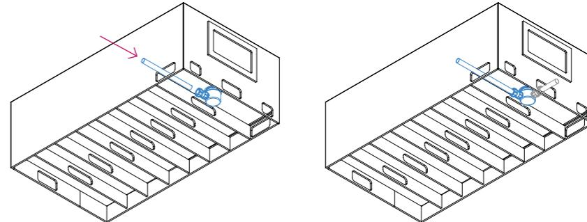
2. Position the base and check level (usually achieved with levelling compound or packers).
