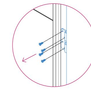
3. Take off side fascias by removing screws. Note the screws on top fascia must also be removed.
