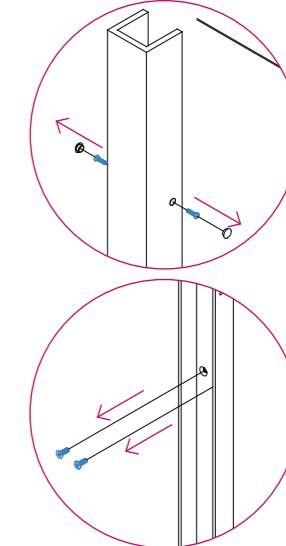
6. Separate soap dishes by removing cover caps and screws.
