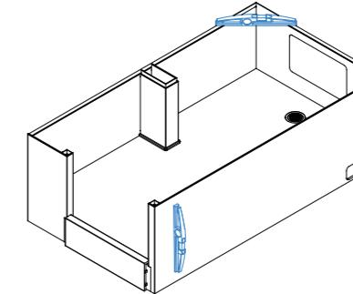
3. Slot in 1<sup>st</sup> middle section and secure with tapping tool and mallet.
