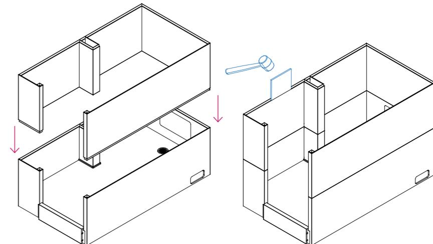
4. Slot in 2<sup>nd</sup> middle section and secure with tapping tool and mallet. Repeat with 3<sup>rd</sup> and 4<sup>th</sup> middle section (if applicable).
