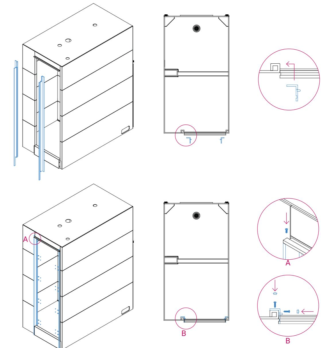
6. Slot in top section and secure with mallet.
