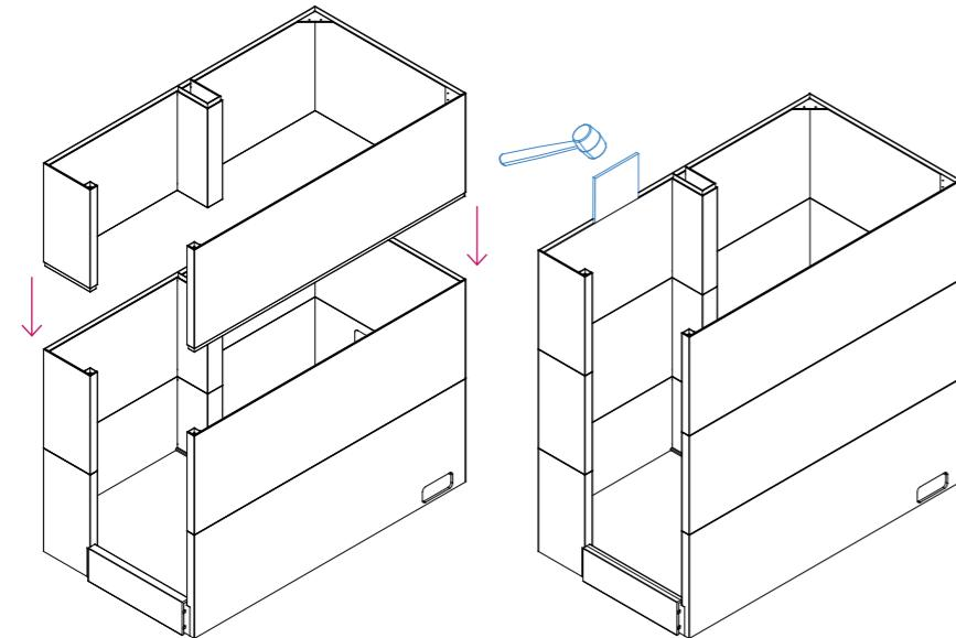
7. Secure top and last middle sections by joining soap dishes with screws and fit cover caps.
