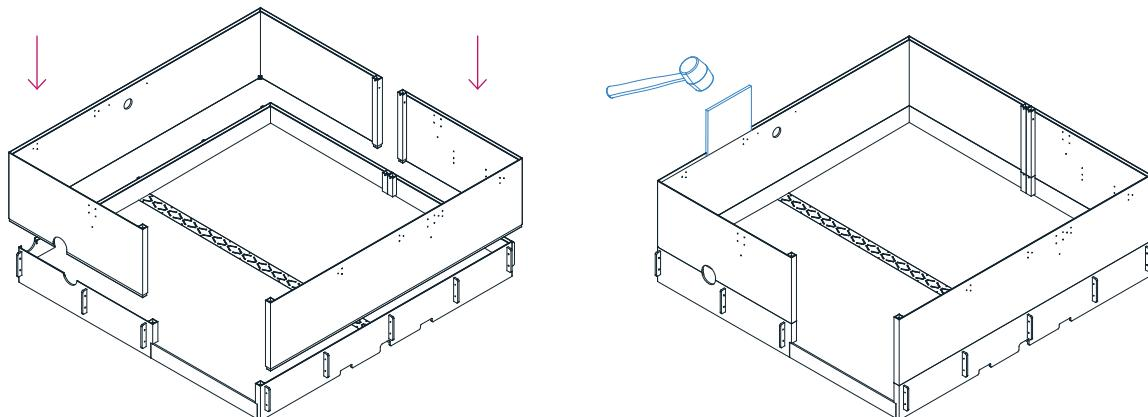
**4.** Use screws to join the back pillar sections from the side.
