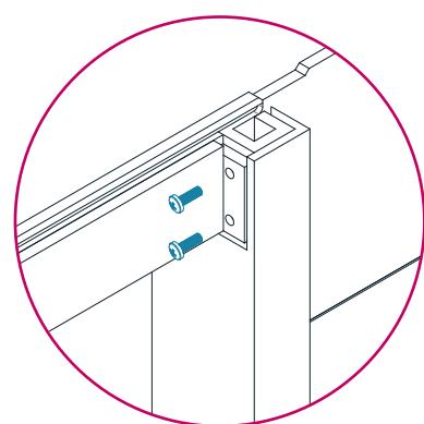
**12.** Secure beam across canopy using the pre fitted 'L' brackets.
