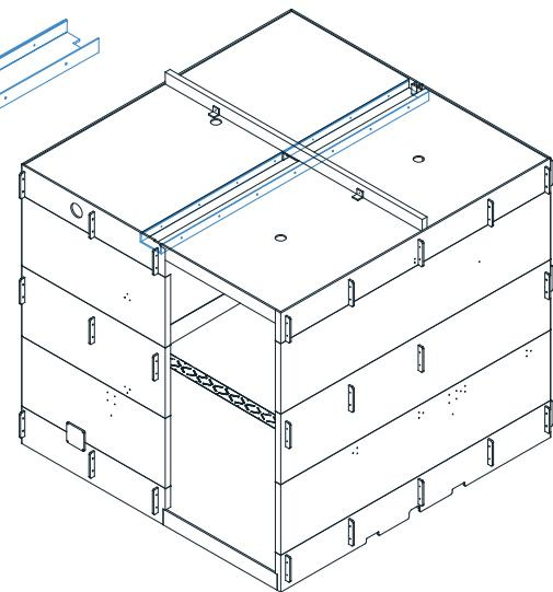
**15.** Use screws and cover caps to fix the pillar cover piece.
