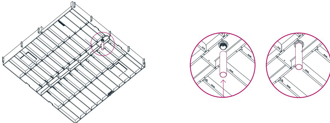
**2.** Position the base and check level (usually achieved with levelling compound or packers).
