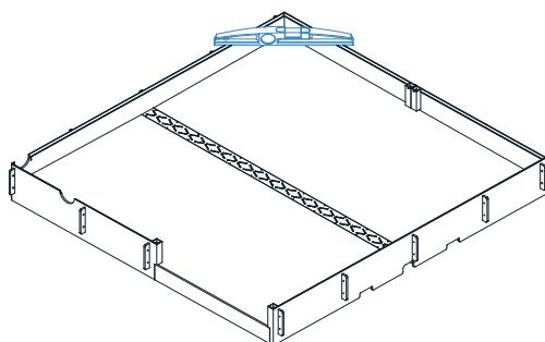
**3.** Slot in the 1" left and right middle sections and secure with tapping tool and mallet.
