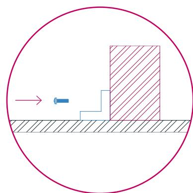
**13.** Align the canopy connecting bracket with the timber beam. Using screws, fix the sides of the bracket into the two parts of the canopy (a.); then the top into the beam (b.).
