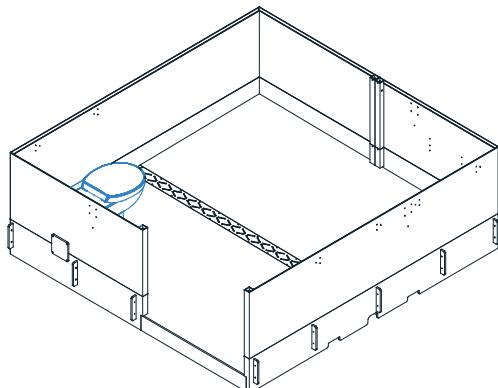
**7.** Slot in the 2<sup>nd</sup> middle sections and secure with tapping tool and mallet.
