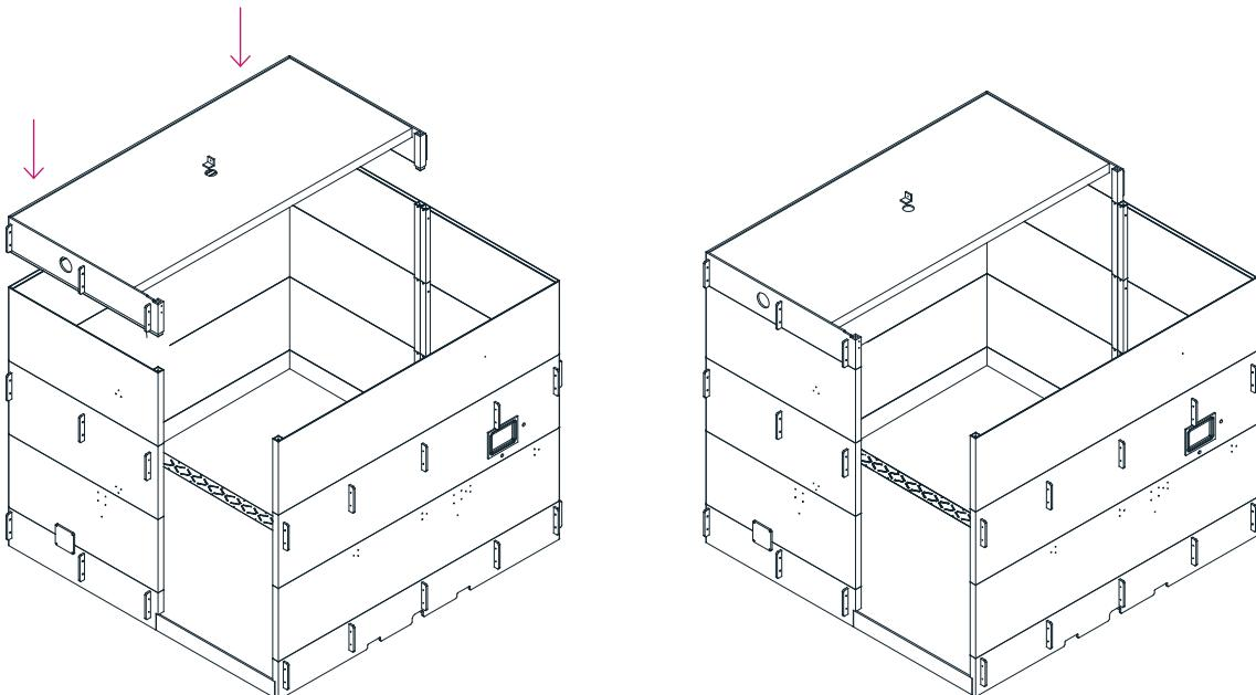
**10.** Slot in wet area canopy (above doorway) and secure with mallet.
