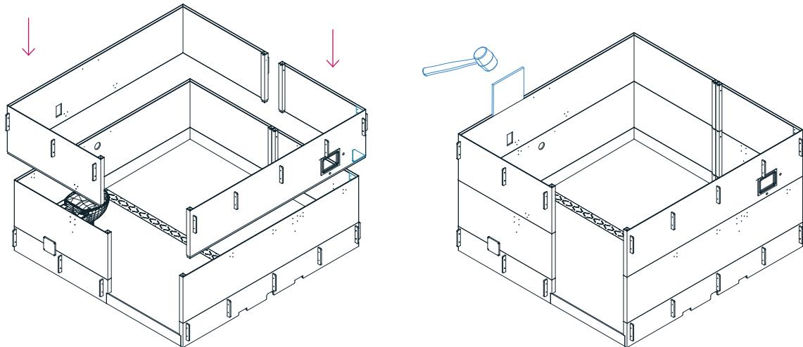
**8.** Secure sections together. Join soap dishes with screws and fit cover caps (a.); use screws to fix back pillars form front and side (b.). Repeat the process with next section.
