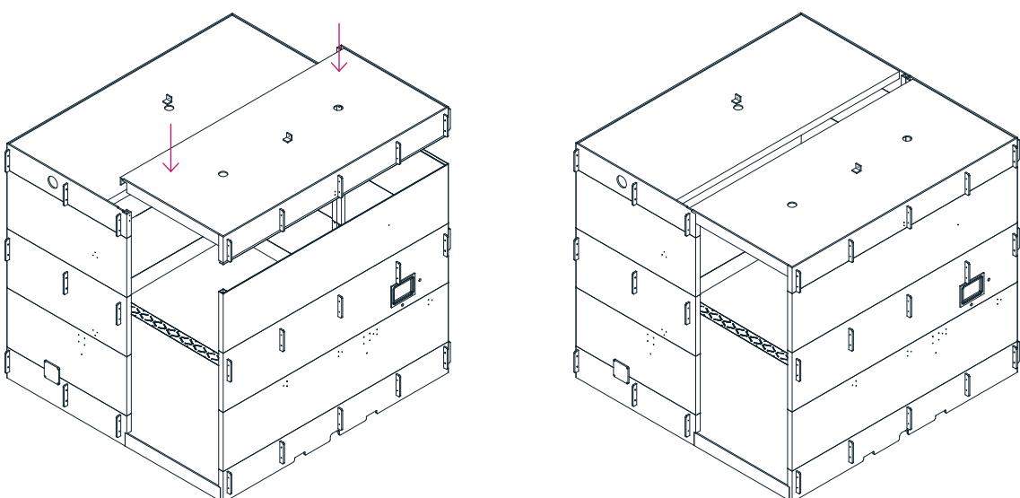
Use screws to join back pillars together from the front and side.
