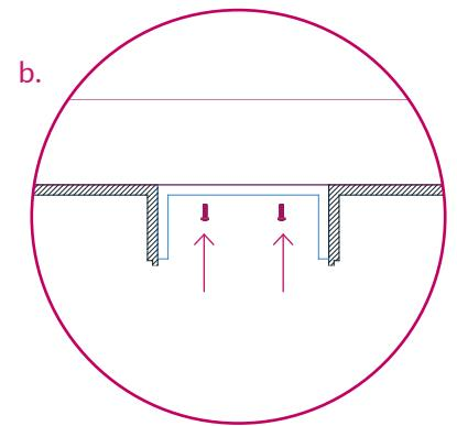
**14.** Slide pelmet into place and secure using screws and cover caps.
