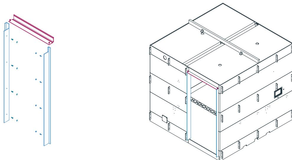
Secure side fascias using screws and cover caps.
