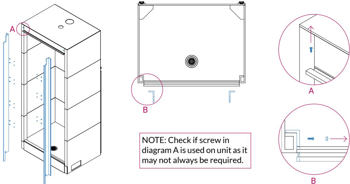
**3. Separate soap dishes by removing cover caps and screws.**
