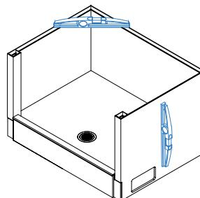
**NOTE:** Ensure that the base is secured in place by fixing it to a wall or to finished floor mounted brackets.
