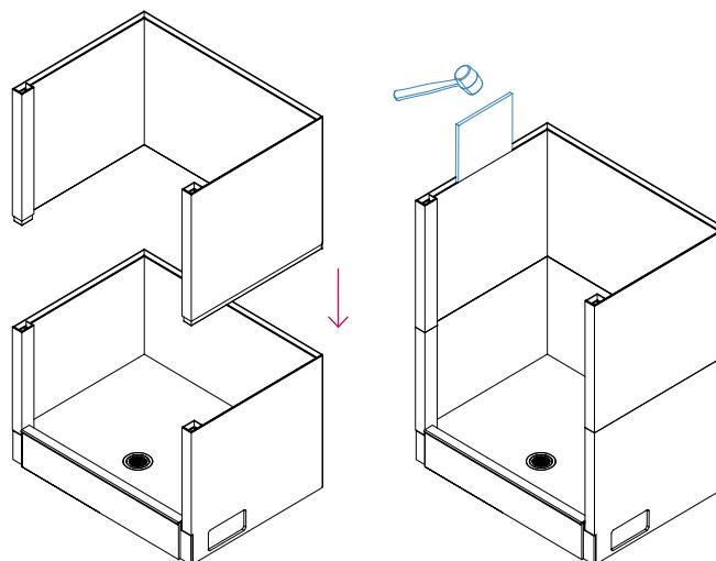
4. Slot in 2nd middle section and secure with tapping tool and mallet. Repeat with 3rd and 4th middle section if applicable.
