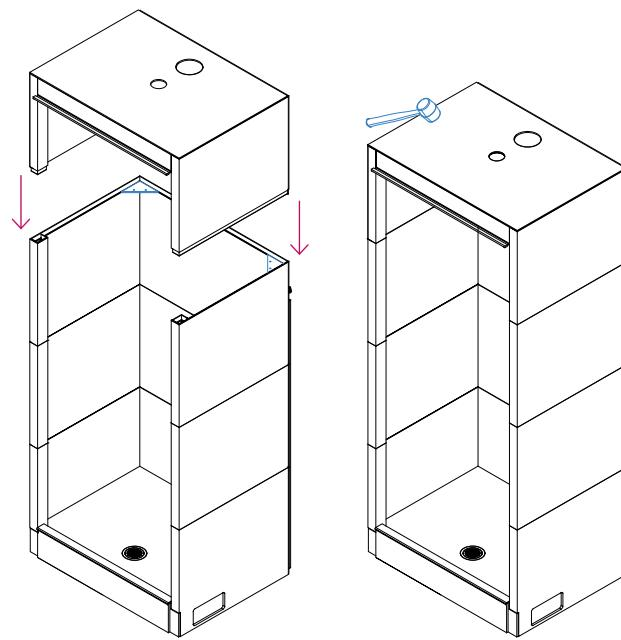
7. Secure top and last middle section by joining soap dishes with screws and fit cover caps.
