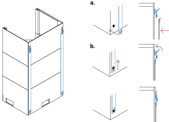
Attach  $\frac{3}{4}$  aluminium backstraps if applicable.
