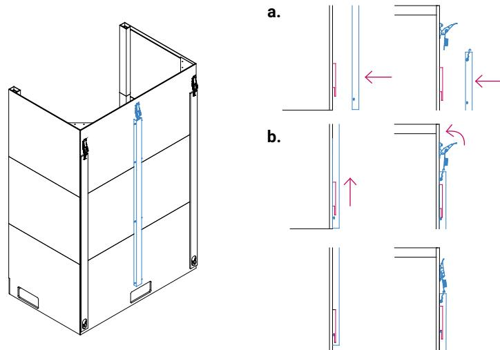
6. Slot in top section and secure with mallet.
