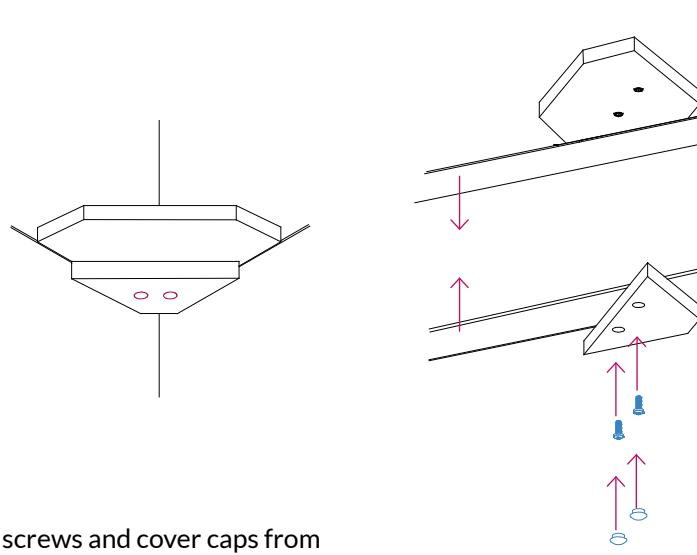
8. Fit side fascias and fix with screws and cover caps from envelope. Be sure to also use previously removed screws. Note the screws on top fascia must also be used.
